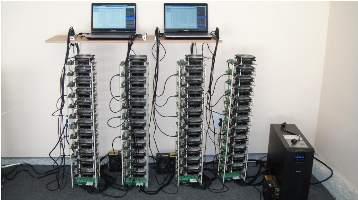
**Figure 5.8: A home-built rack of FPGAs.** Although you don't see the cooling setup pictured here, a rack like this would need a cooling system.
